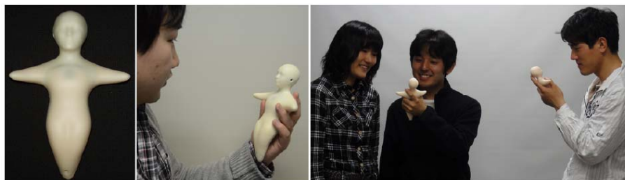
FIGURE 1. Cell phone-type tele-operated android robot “Elfoid”™
