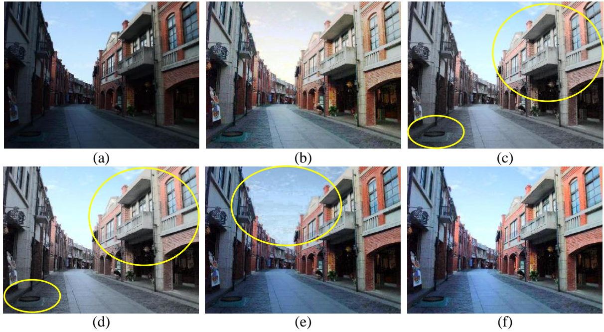
FIGURE 3. The “Street” color image: (a) is the original image; the remaining five images are the enhanced images using HE with (b) RGB color model [26], (c) G channel of RGB [24], (d) YUV color model [28], (e) HSV color model [27] and (f) spherical color model
