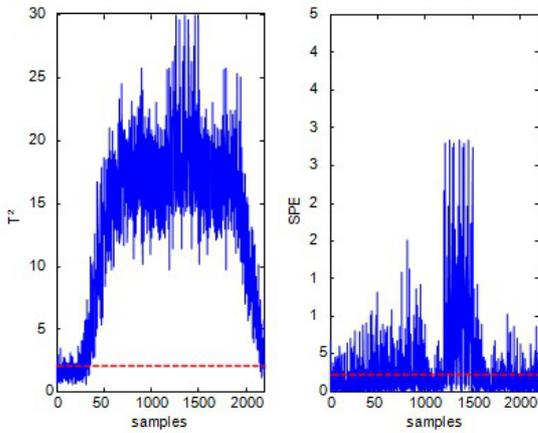
FIGURE 6. Monitoring by DPCA with conventional indices
