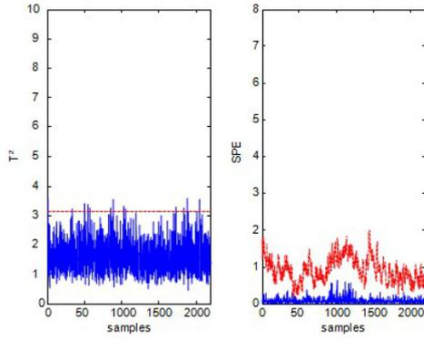
FIGURE 4. Normal variations by recursive DPCA (fault free) with conventional indices
