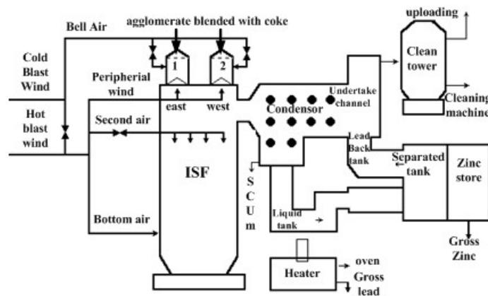
FIGURE 1. Imperial smelting furnace structure
