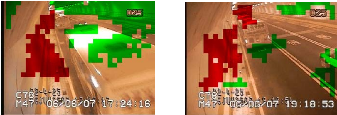
FIGURE 16. False alarms caused by exposure adjustment (Red indicates blocks with smoke and green indicates non-smoke blocks)
