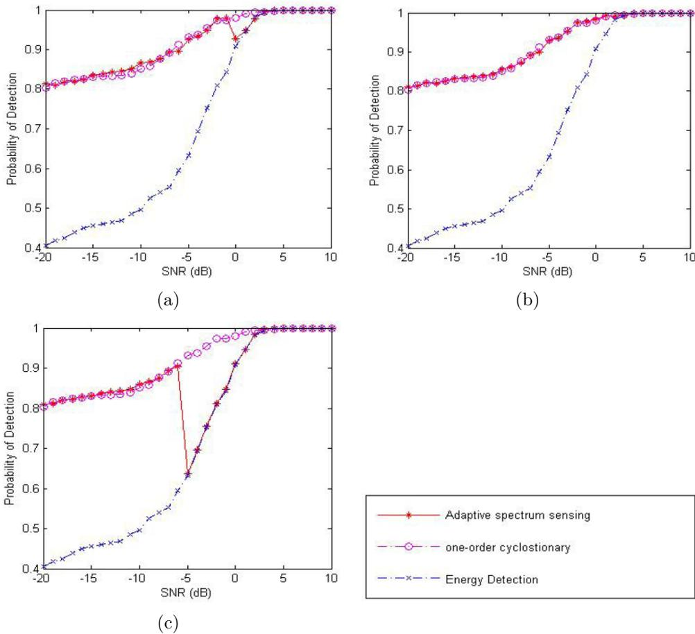
FIGURE 5. Detection performance versus SNR comparison of proposed adaptive spectrum sensing, one-order cyclostationary detector and energy detector for thresholds (a)  $\lambda = 0$ , (b)  $\lambda = 5$ , and (c)  $\lambda = -5$
