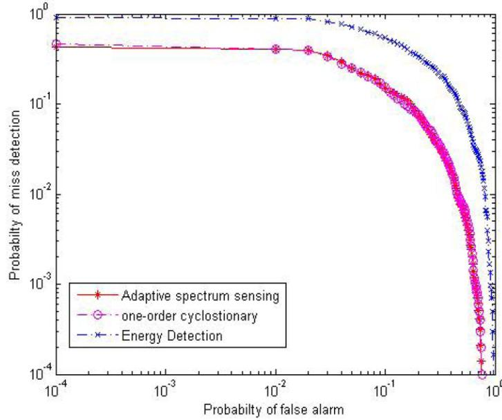
FIGURE 4. ROC curves of proposed adaptive spectrum sensing, one-order cyclostationary detection and energy detection
