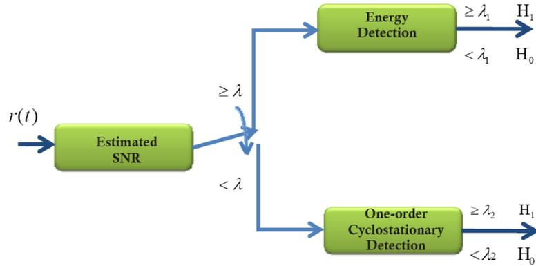
FIGURE 1. Adaptive spectrum sensing scheme
