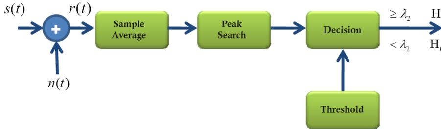
FIGURE 3. Block diagram of one-order cyclostationary detection [14]
