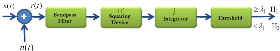
FIGURE 2. Block diagram of energy detection
