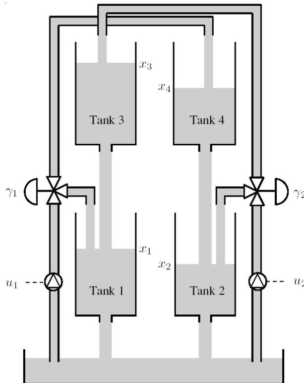
FIGURE 1. Schematic diagram of the quadruple-tank system
