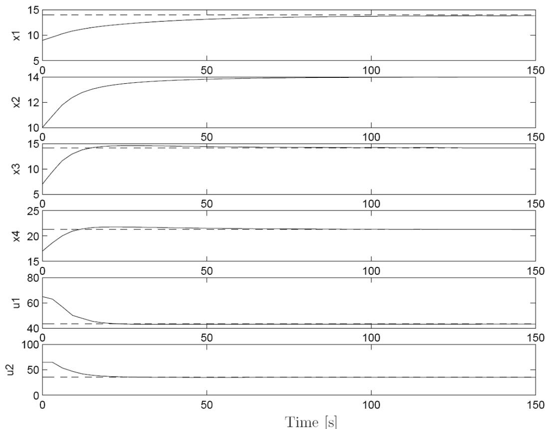
FIGURE 3. Simulation results with C/GMRES: setpoint (dash-dotted), simulation (solid)
