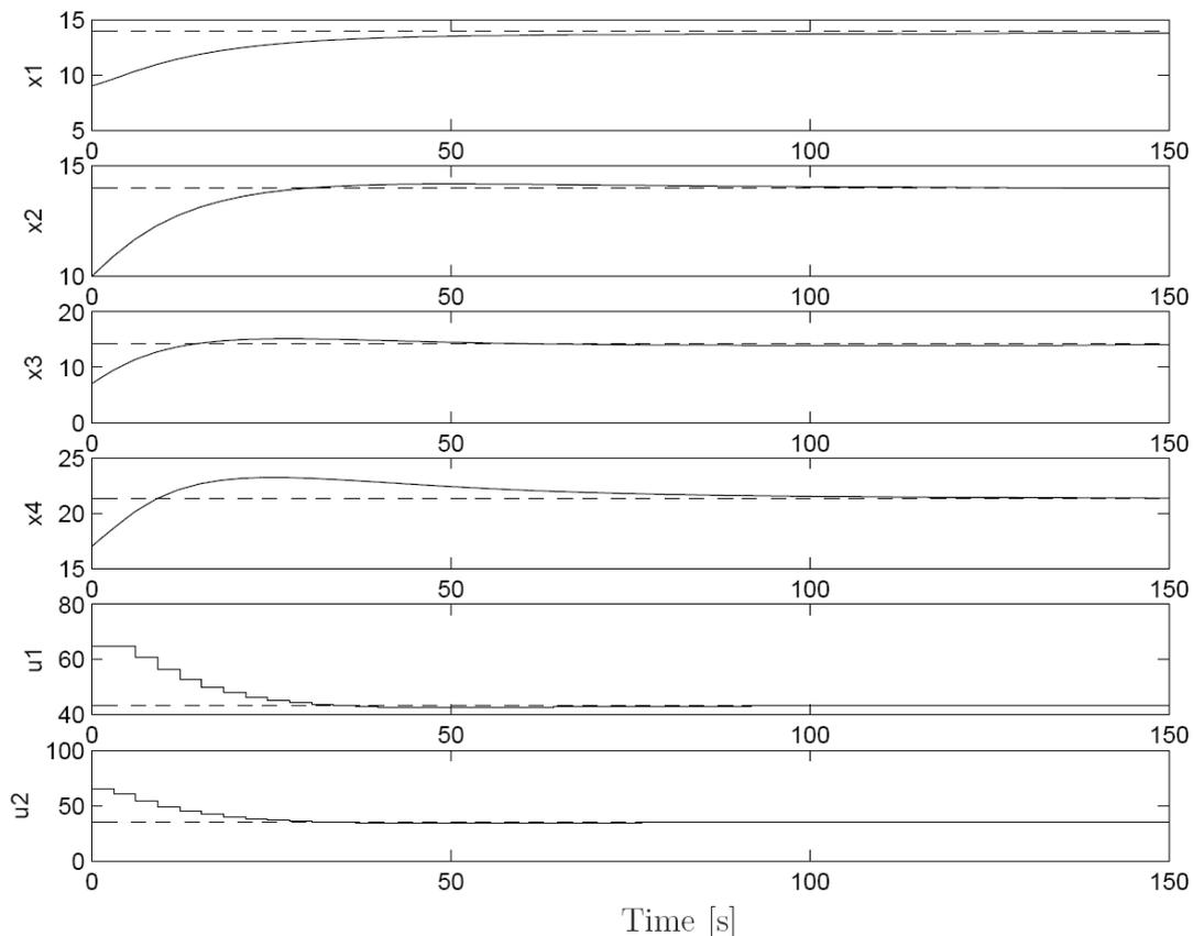
FIGURE 2. Simulation results with quasi-infinite horizon NMPC: setpoint (dash-dotted), simulation (solid)
