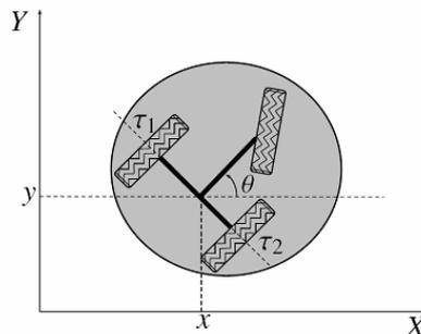
FIGURE 2. Diagram of a wheeled mobile robot
