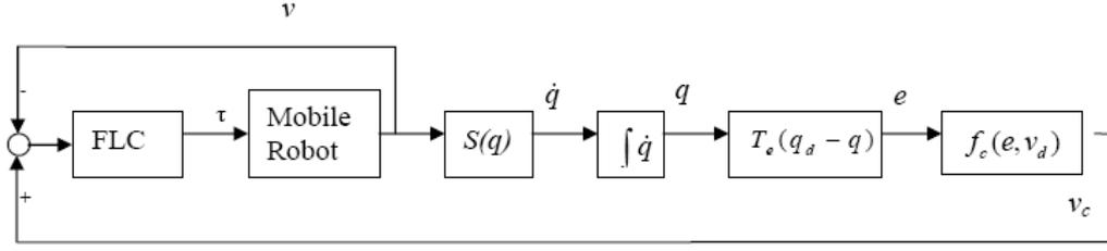
FIGURE 3. Tracking control structure
