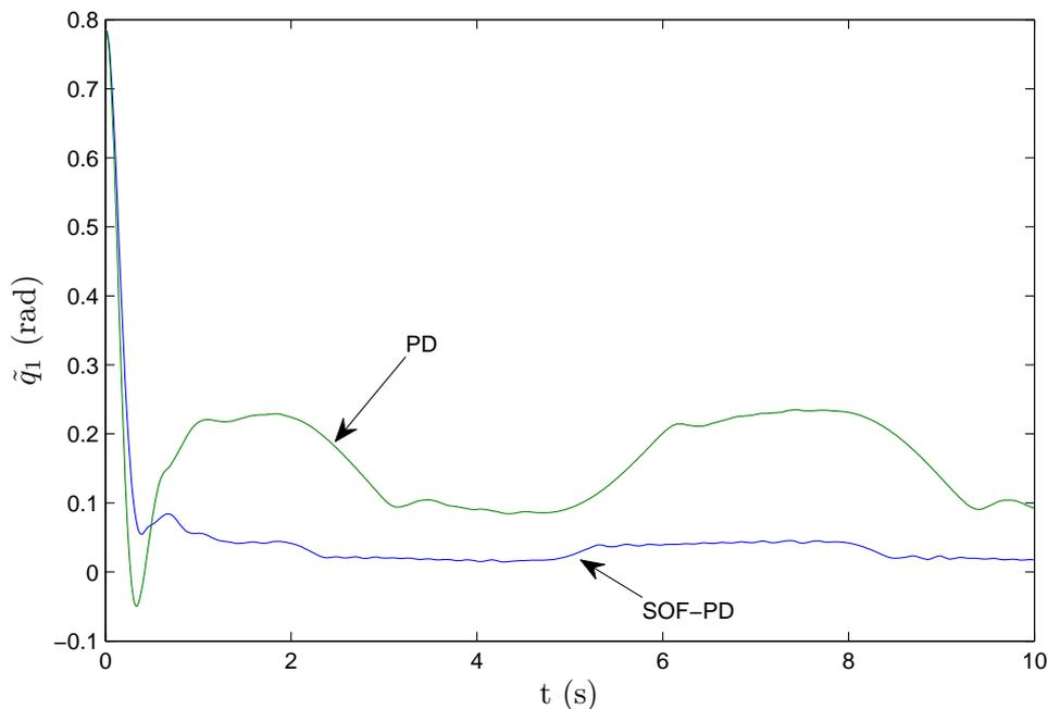
FIGURE 4. Tracking errors on  $q_1$
