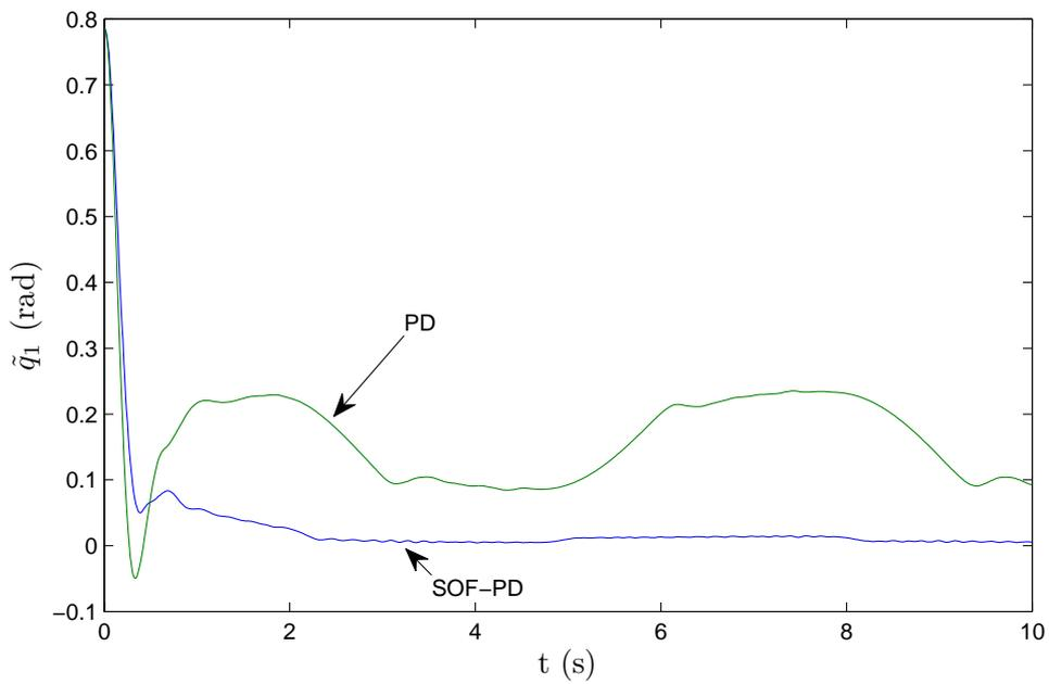
FIGURE 11. Tracking errors on  $q_1$  with the new tuning of the SOF-PD
