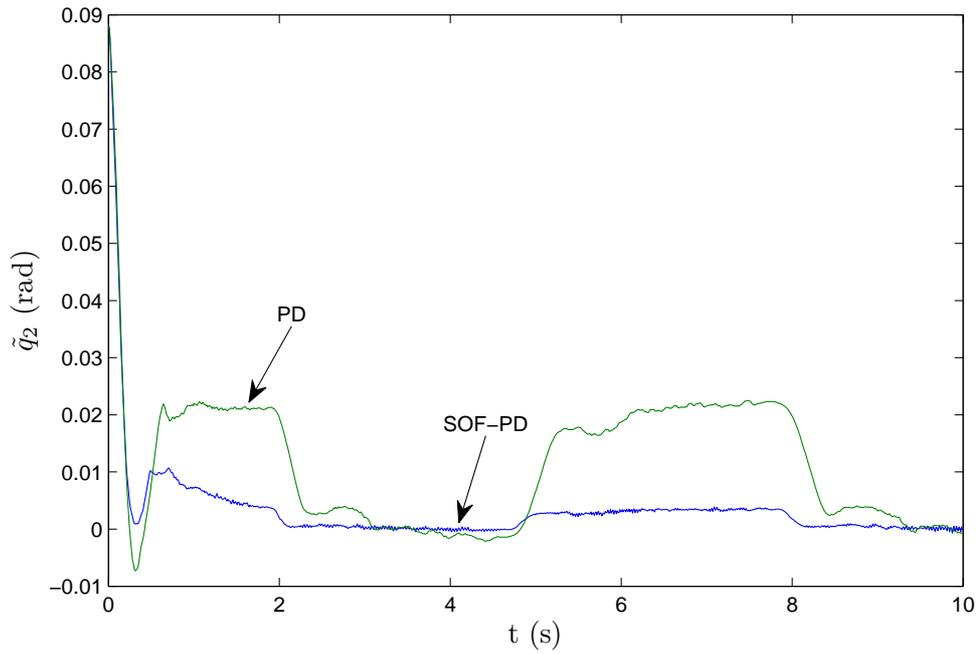
FIGURE 5. Tracking errors on  $q_2$
