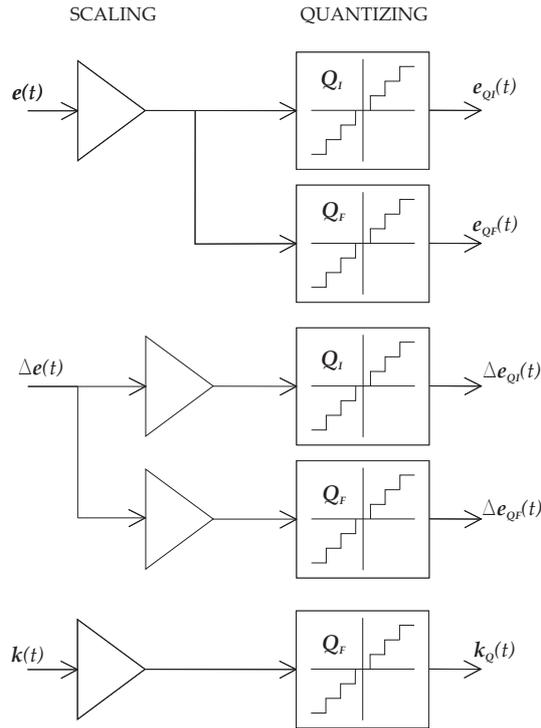
FIGURE 2. SOF input section
