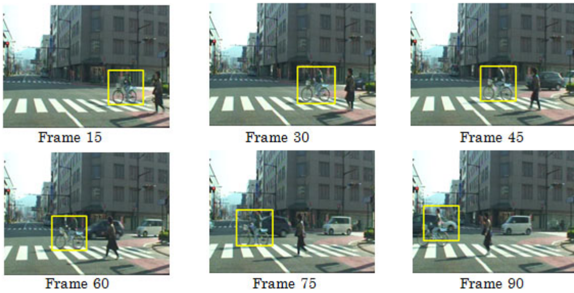
FIGURE 6. Result of Exp_1v1: Detection of a bicycle – The case where there is no occlusion with the bicycle
