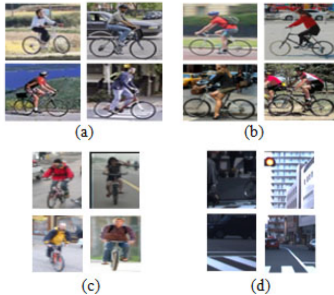
FIGURE 5. Samples of the employed training data: (a) right direction, (b) left direction, (c) front direction, (d) background
