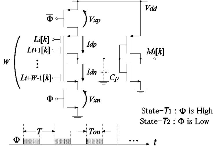
FIGURE 3. Majority circuit using a clocked neuron CMOS inverter
