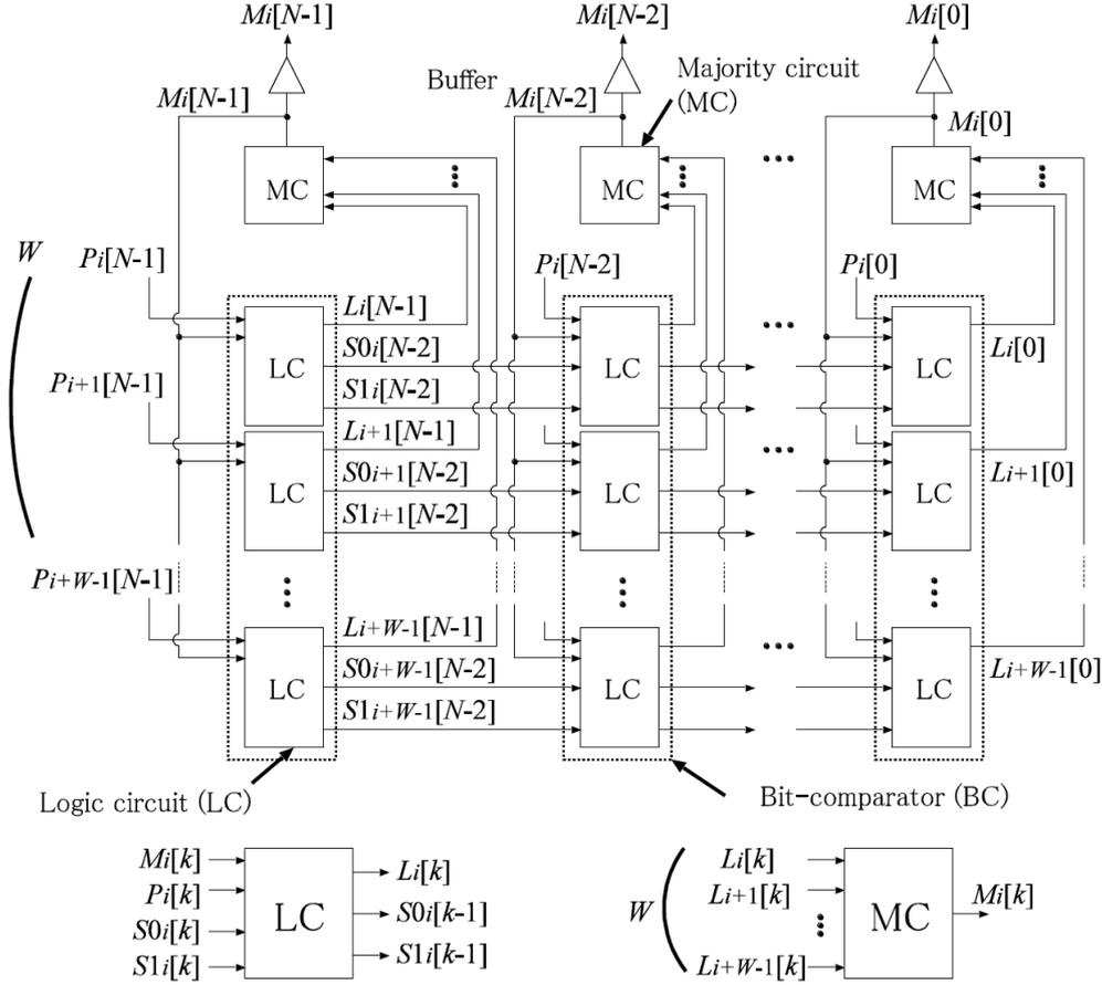
FIGURE 1. Block diagram of CMOS median filter
