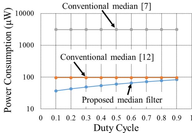
FIGURE 5. Simulated power consumption of the median filter
