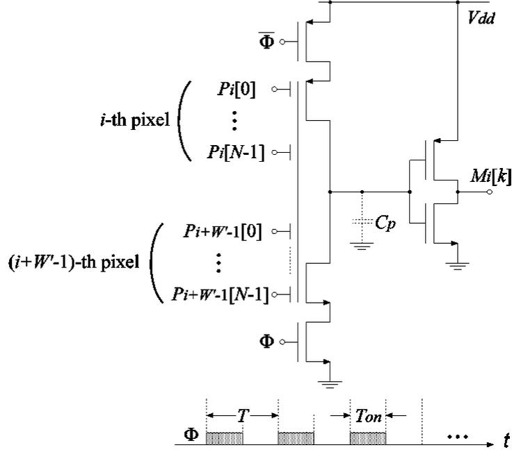
FIGURE 7. Binarizing and resizing circuit using a clocked neuron CMOS inverter
