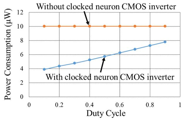
FIGURE 9. Simulated power consumption of the median filter
