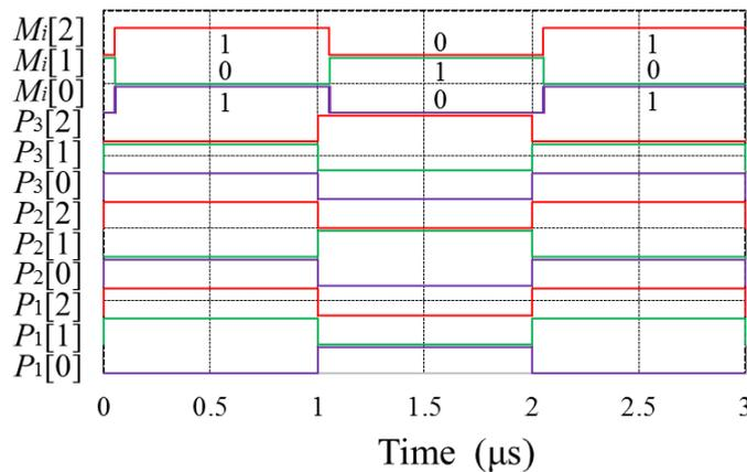
FIGURE 4. Simulated output of the proposed median filter
