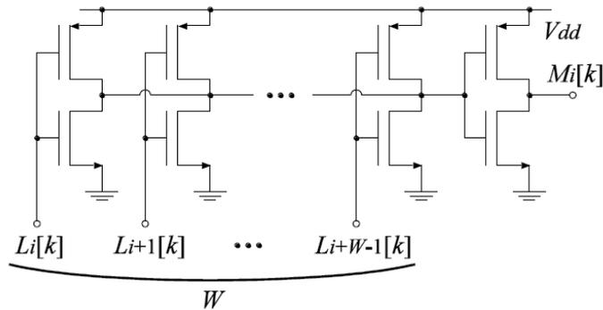
FIGURE 6. Conventional CMOS majority circuit [7]
