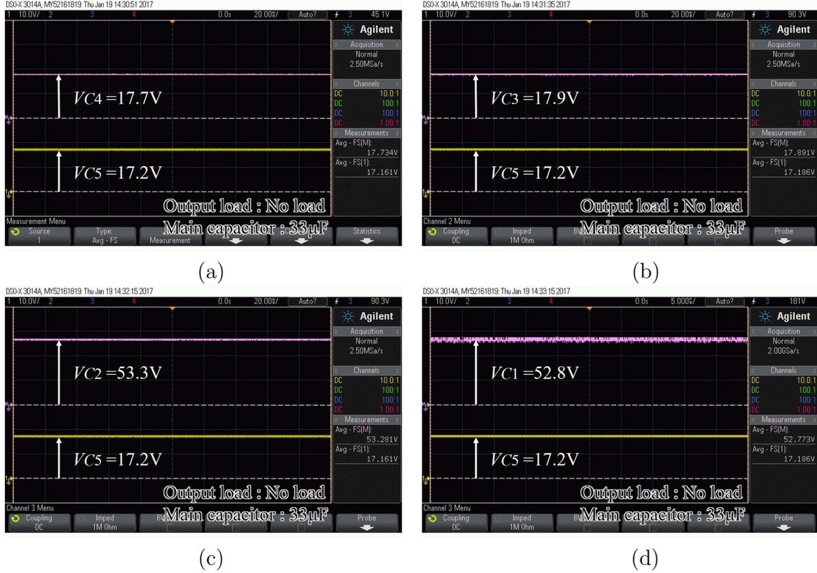
FIGURE 11. Measured voltage of capacitors; (a)  $C_5$  vs.  $C_4$ , (b)  $C_5$  vs.  $C_3$ , (c)  $C_5$  vs.  $C_2$ , and (a)  $C_5$  vs.  $C_1$
