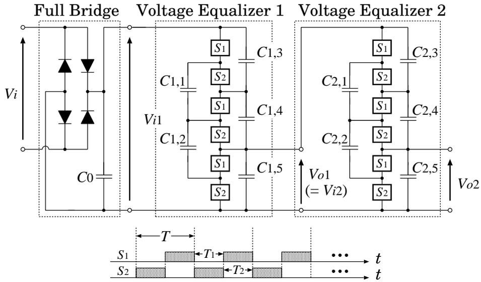
FIGURE 1. Conventional SC ac/dc converter proposed in [12]
