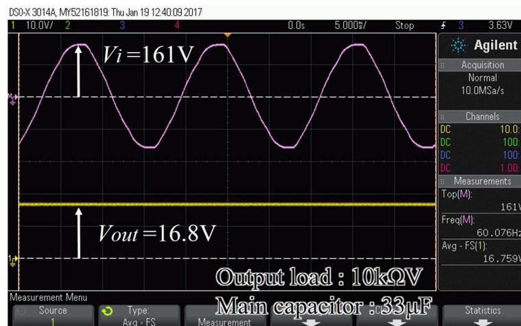
FIGURE 10. Measured output voltage of the experimental circuit
