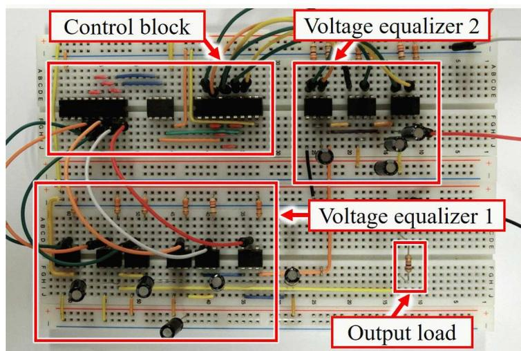
FIGURE 9. Experimental circuit of the proposed converter
