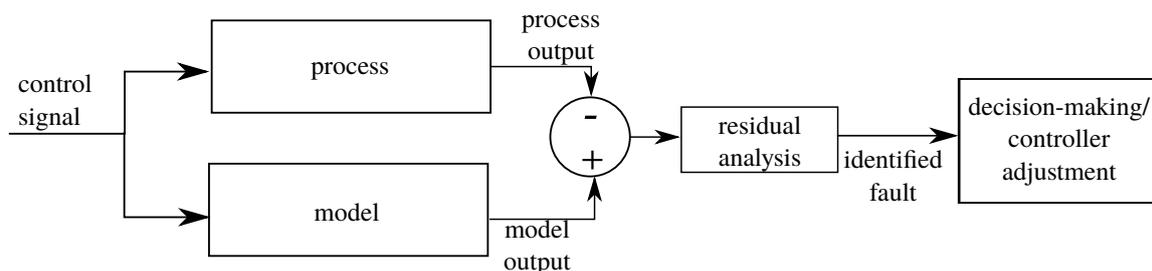
FIGURE 1. Model-based fault identification and treatment system based on [7]
