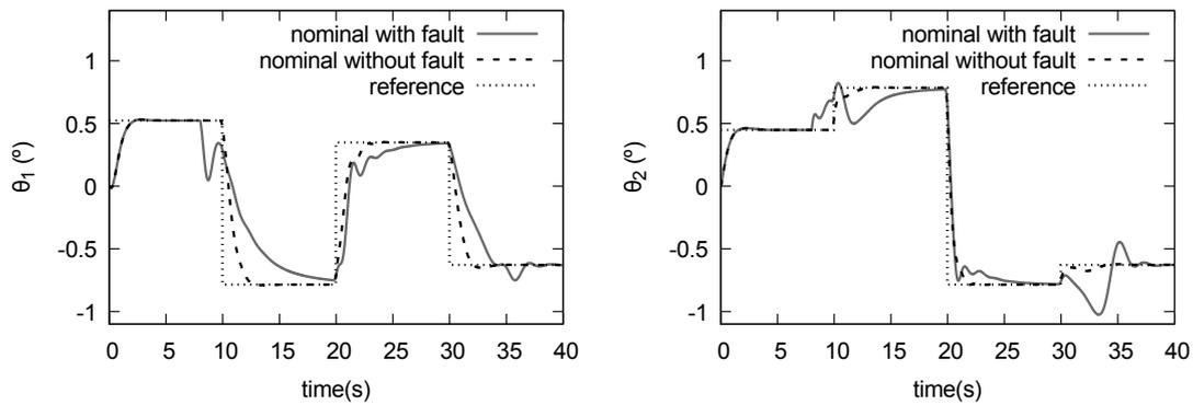
FIGURE 5.  $\theta_1$  and  $\theta_2$  responses with nominal FCC-NMPC with and without the fault
