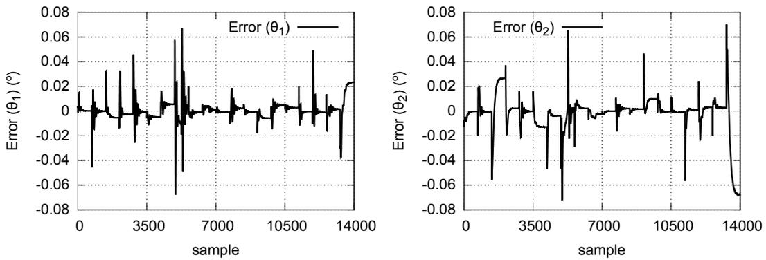
FIGURE 4.  $\theta_1$  and  $\theta_2$  validation errors between the trained FCC-ANN and the simulated model
