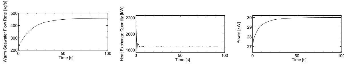
FIGURE 6. Simulation result ( $m_{WS}$  is regulated by PI controller for  $T_{WSI} = 29$  [°C] (constant))
