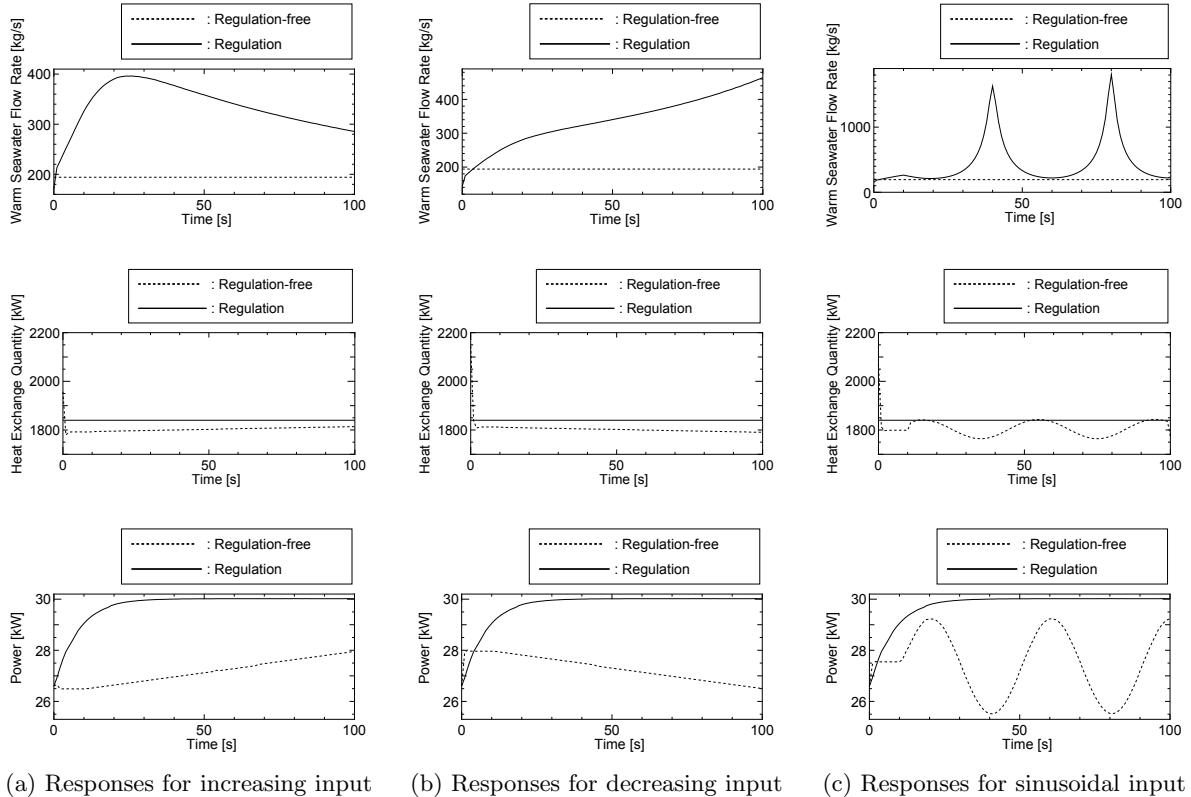
FIGURE 7. Simulation results (regulation of  $m_{WS}$ )
