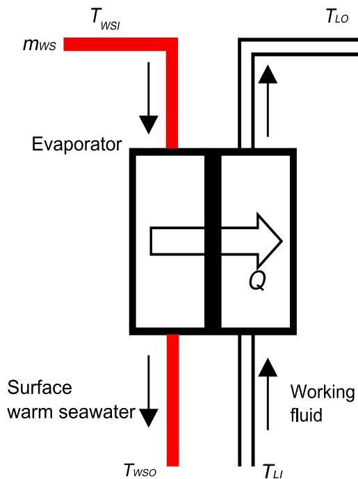
FIGURE 2. Heat exchange in evaporator
