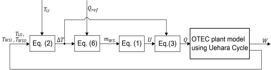
FIGURE 3. Block diagram of warm seawater flow rate regulation
