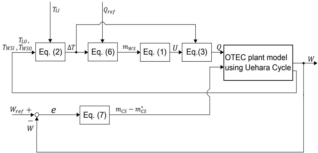
FIGURE 4. Block diagram of warm and cold seawater flow rate regulation
