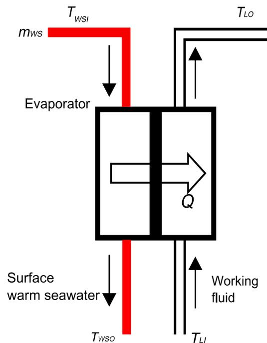
FIGURE 2. Heat exchange in evaporator
