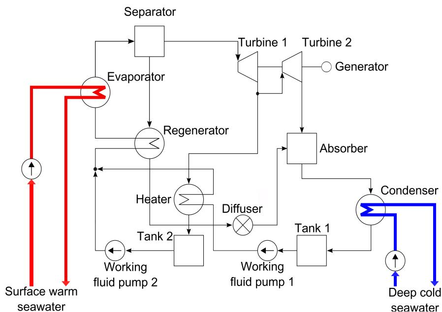
FIGURE 1. Overview of OTEC plant using Uehara cycle
