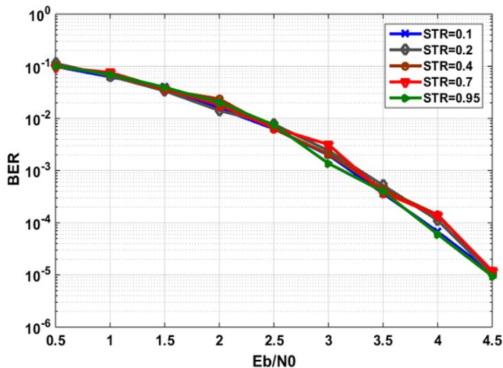
FIGURE 9. Impact of the parameter STR on S2W2Dec performances for QR(71, 36)
