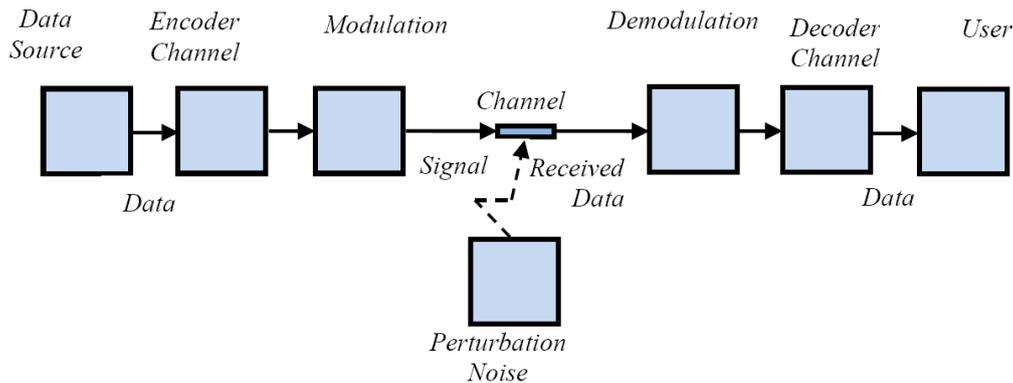
FIGURE 1. A simplified model of communication systems
