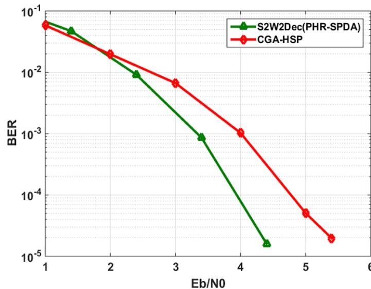
FIGURE 16. Comparison between BER performances of CGA-HSP and S2W2Dec(PHR-SPDA) for QR(71, 36) code
