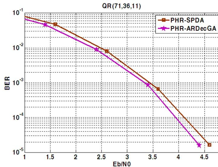
FIGURE 11. Comparison of BER performances of S2W2Dec(PHR-SPDA) and S2W2Dec(PHR-ARDecGA)
