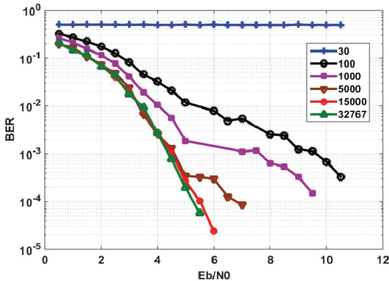
FIGURE 2. Impact of the number  $M$  of dual codewords on the PHR performances for the QR(31, 16, 7) code
