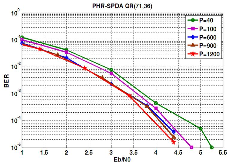
FIGURE 6. Impact of the permutations number  $P$  on S2W2Dec(PHR-SPDA) performances
