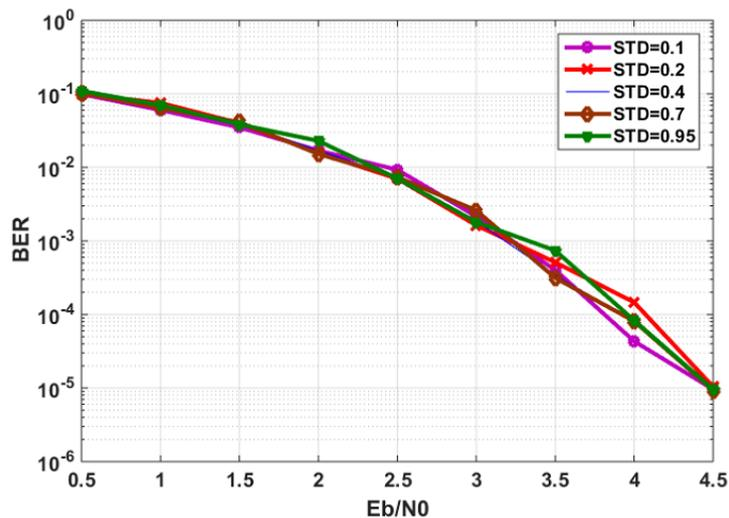
FIGURE 10. Impact of the parameter STD on S2W2Dec performances for QR(71, 36)
