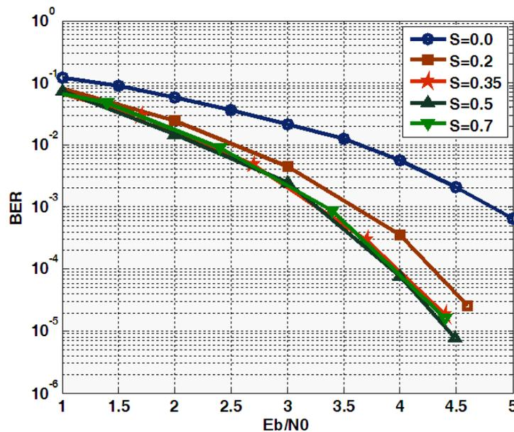
FIGURE 8. Impact of the parameter  $S$  on S2W2Dec performances for QR(71, 36) code
