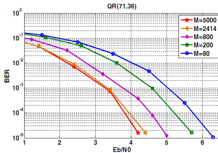
FIGURE 7. Impact of the parameter  $M$  on S2W2Dec performances for QR(71, 36) code
