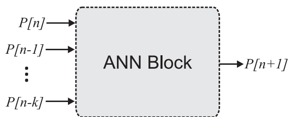
FIGURE 6. Artificial neural network for forecasting the next value. The window used was 10 samples ( k = 9 ).
