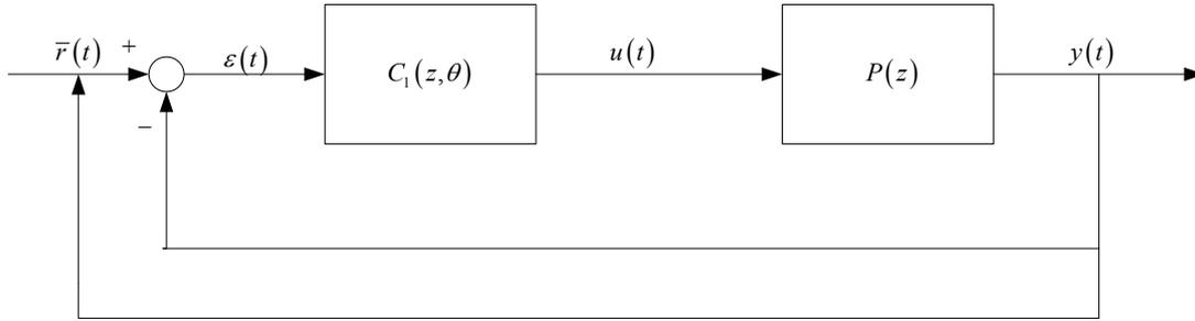
FIGURE 2. Construction of virtual input
