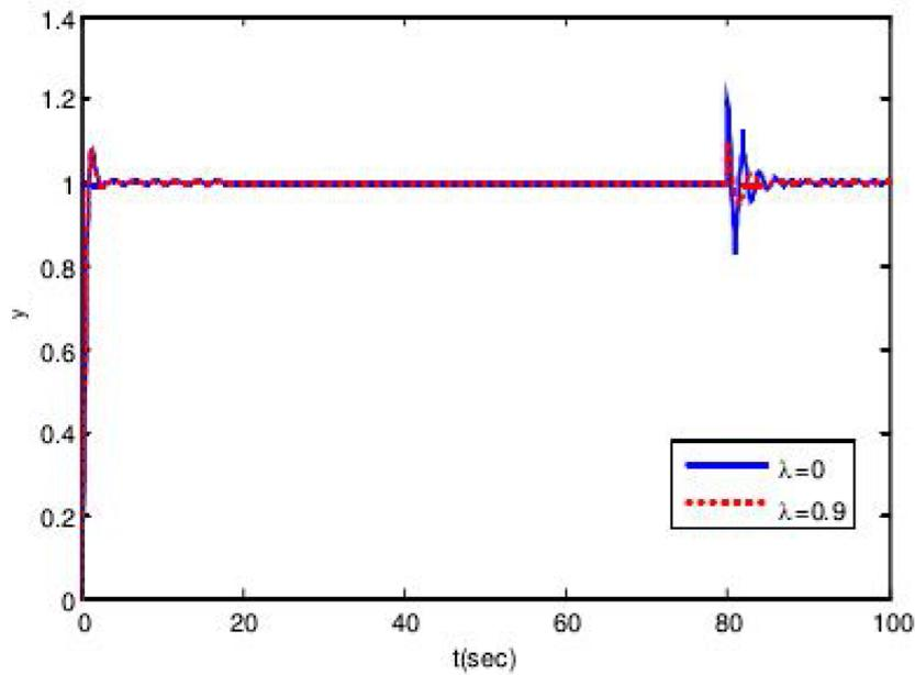
FIGURE 5. Step response curve for adaptive direct data driven control
