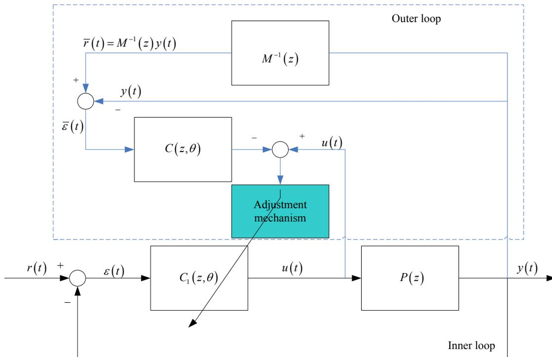
FIGURE 3. Block diagram of adaptive direct data driven control scheme
