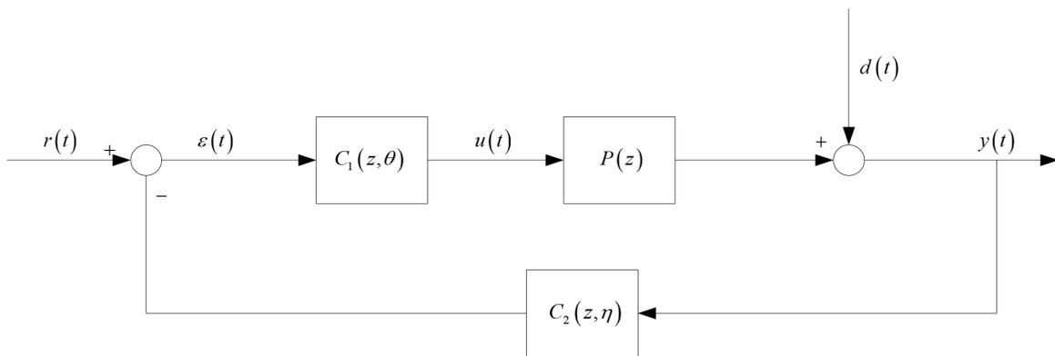
FIGURE 9. Closed loop system with two degrees of freedom controllers
