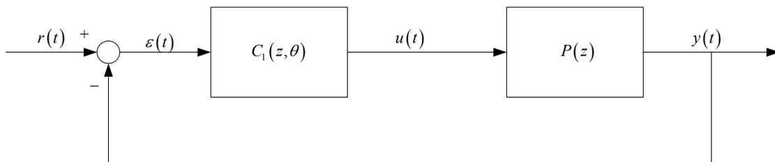
FIGURE 1. Closed loop system structure
