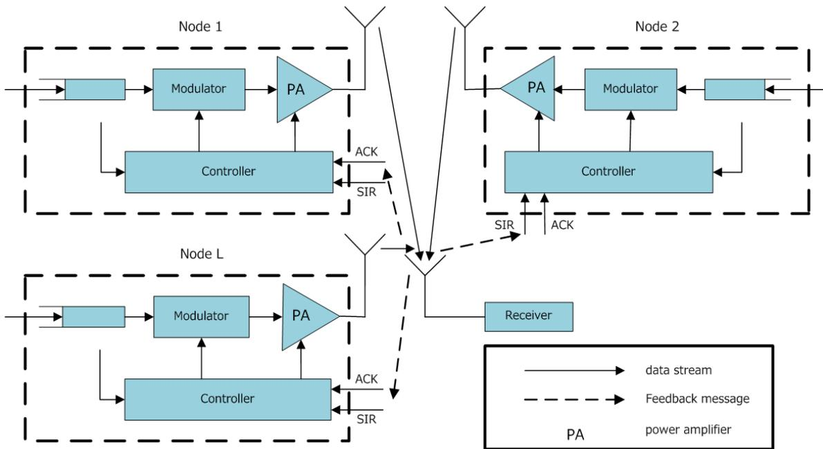
FIGURE 2. Multi-node communication mode
