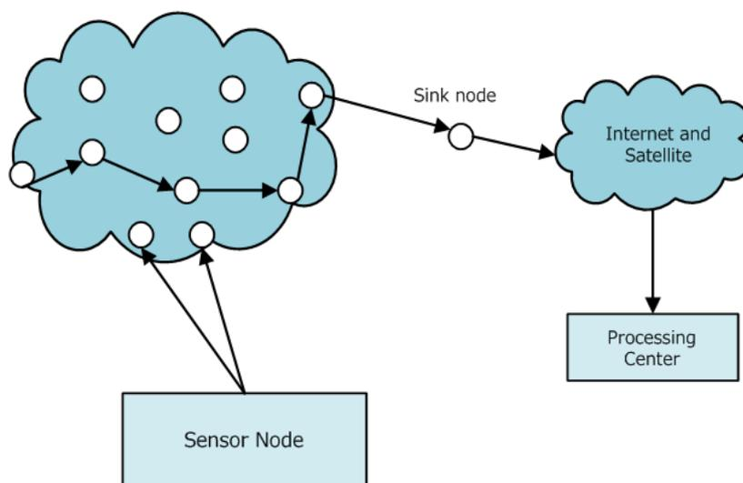
FIGURE 1. Composition of wireless sensor networks
