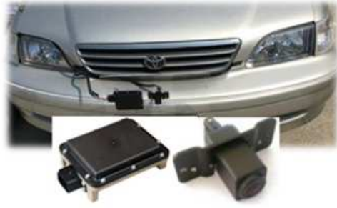
FIGURE 2. The sensors installation
