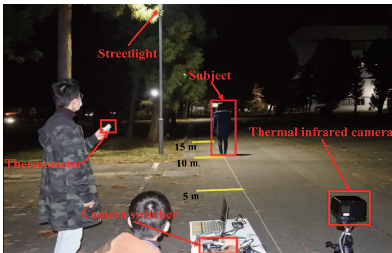
FIGURE 5. Data-acquisition environment (streetlight on; low temperature; subject standing)
