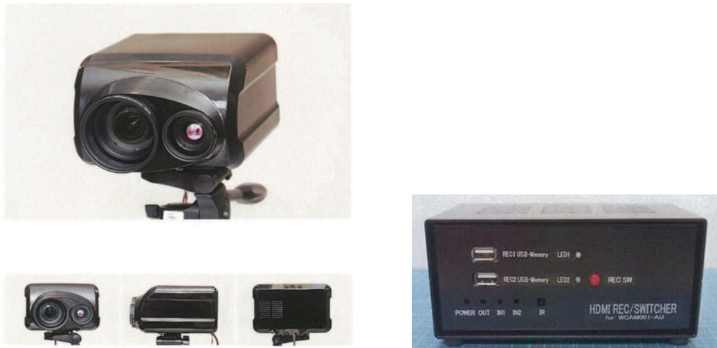
FIGURE 4. External view of the infrared thermal imaging camera and switcher (standard type)
